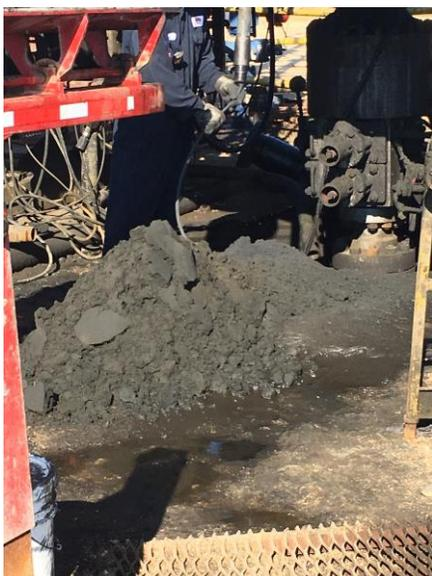
With the VACS G2 system, 7.8 barrels of scale (iron sulfide, calcium carbonate, and frac sand) was recovered from the wellbore in six runs, resulting in a production increase of 700 B/D.
