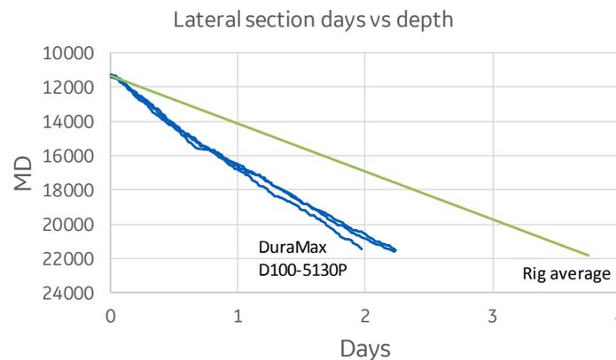
Navi-Drill DuraMax reduced drilling time by 40%. MD illustrates the measured depth in feet.
