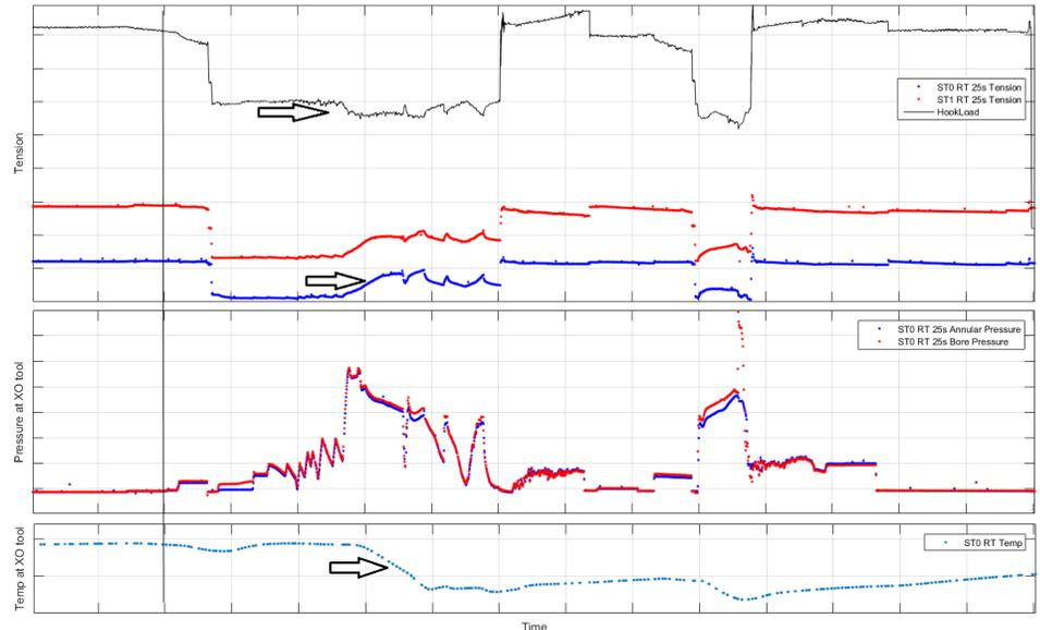
Real-time results transmitted during the completion installation process. The arrows indicate when cooler fluids were pumped down the string. The bottom light blue curve is the temperature downhole at the crossover tool. As the temperature cooled, over 70 klb came off the packer due to contraction of the string. Surface data indicated in error only a 20 klb reduction.
