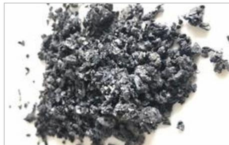
Because the MILLITE lightweight frac plug is built completely out of a special lightweight alloy that is 70% lighter than conventional plug material, it produced smaller cuttings that were much easier to circulate, leaving less debris in the well.
