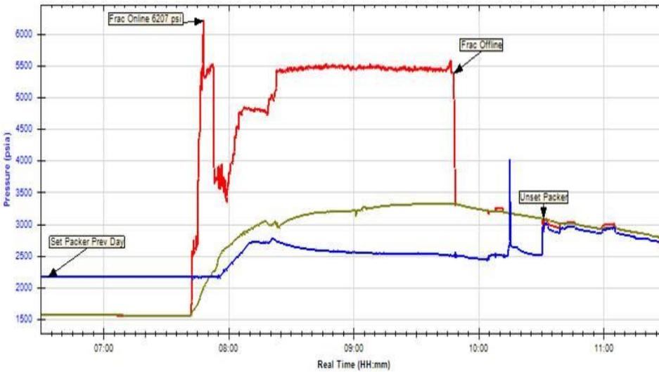
Recorded data from memory gauges during the refracture treatment. Red is the injection pressure into the formation. Blue is below the packers. Green is above the packers.
