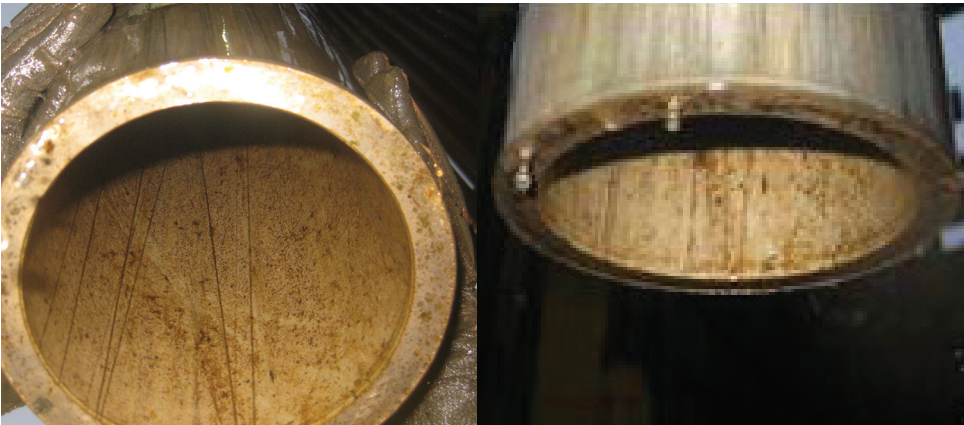
Tubing after being pulled to surface.
