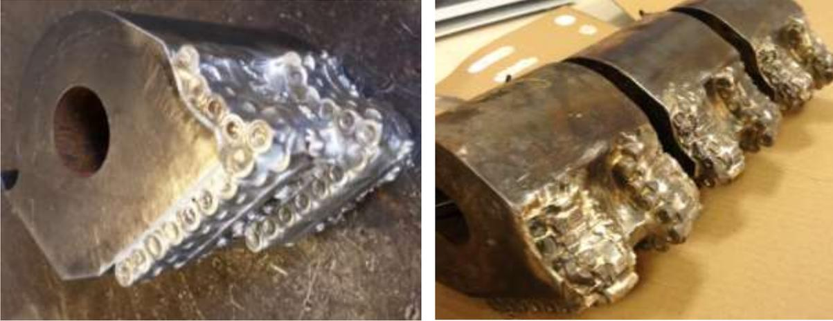
Figure 1. Comparison of new knife (left) and used knives (right) after 17 cuts, showing minimal wear of METAL MUNCHER AMT inserts.
