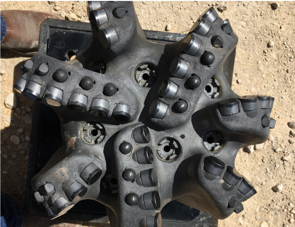
The Dynamus bit had almost no damage or wear after drilling the longest run in the interval
