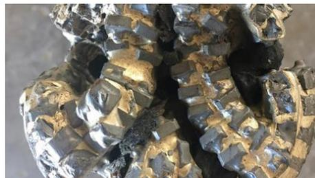
Condition of Glyphaloy-dressed mill after milling 72 composite frac plugs in a single run.
