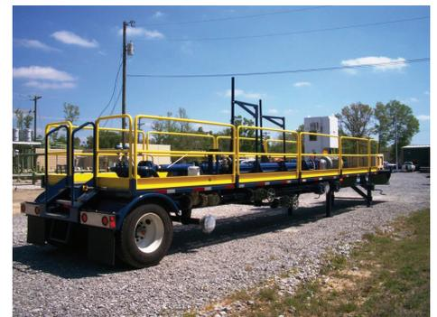
BHGE CO<sub>2</sub> trailer-mounted horizontal surface pumping system.
