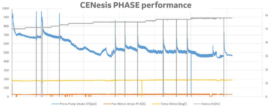
CENesis PHASE performance in a well with high gas content in the fluid stream.
