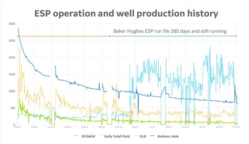
Historical production and operation data of the well with the run life of a competitor's ESP system on the left and the performance of the CENesis PHASE solution on the right
