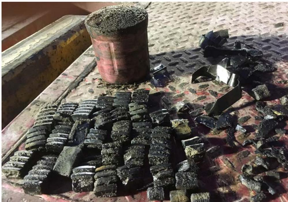
Eight joints of tubing filled with sand, 28 cast iron slips, two ESP monel bands, and a handful of miscellaneous plug parts were recovered in just one trip.
