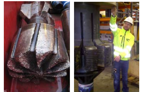
A specialized 18 5 / 8 -in. METAL MUNCHER AMT junk mill was used to mill the seal assemblies.
