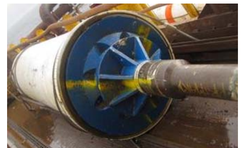
The 42-in. washout sleeve on deck after successful removal using a modified HERCULES casing cutter and Model E spear.
