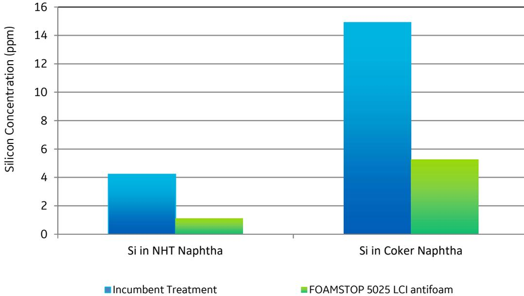
Figure 1. Silicon (Si) concentrations in both the NHT naphtha and coker naphtha were significantly reduced when using FOAMSTOP 5025 LCI antifoam compared to the incumbent product.
