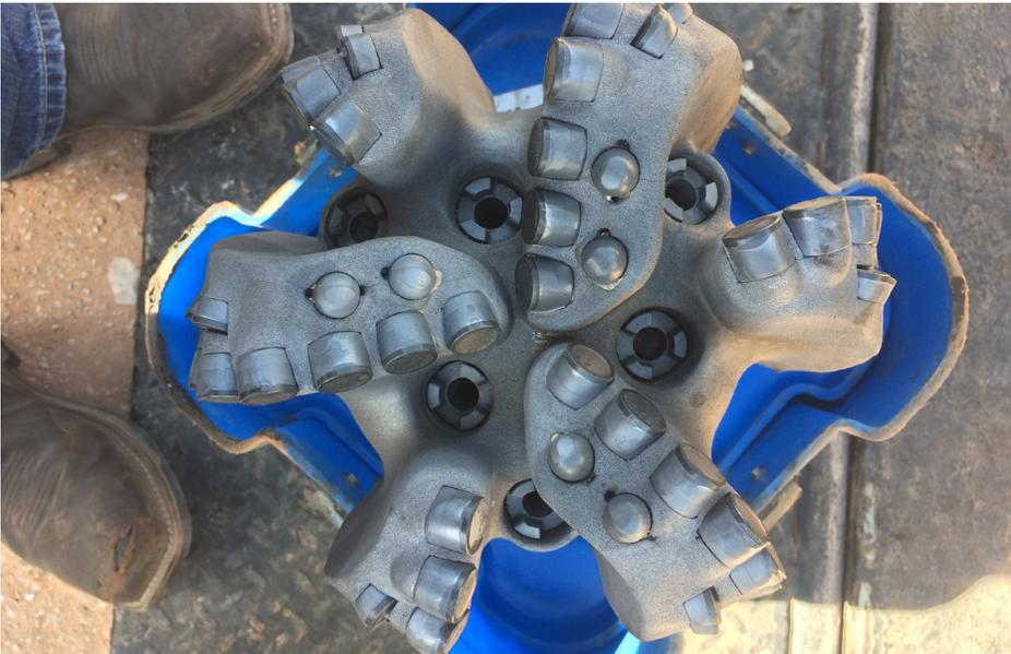
After the Dynamus bit drilled the entire lateral in one run, it was in nearly perfect condition with minimal wear or damage.
