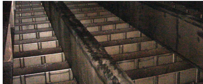
Vacuum tower vortex breaker (above) are clean and debris free after a combined liquid circulation/vapor phase decontamination. Crude tower wash trays (below) after a vapor phase decontamination only.
