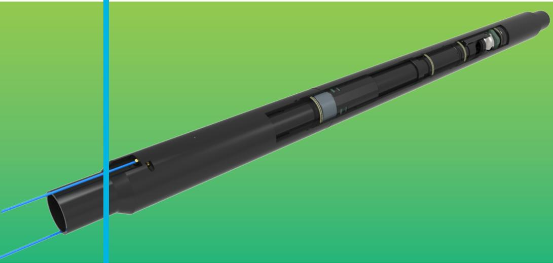
The Caledyne Hydraulic Ball Valve (HBV) delivers reliable isolation between the upper and lower completion and enables interventionless opening and closing via hydraulic control lines, saving rig time and reducing OPEX. When sufficient lubricator height is not available, the HBV can also isolate the well and create a lubricator section, allowing longer strings to be installed.
