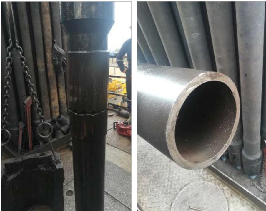
The first image shows the failed pipe cut attempted by another wireline company; the second image shows the precise cut made by the BHGE MPC
