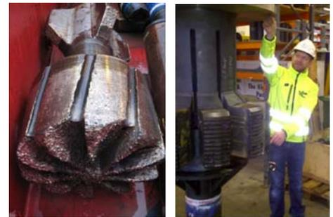
A specialized 18<sup>5</sup>/<sub>8</sub>-in. METAL MUNCHER AMT junk mill was used to mill the seal assemblies.
