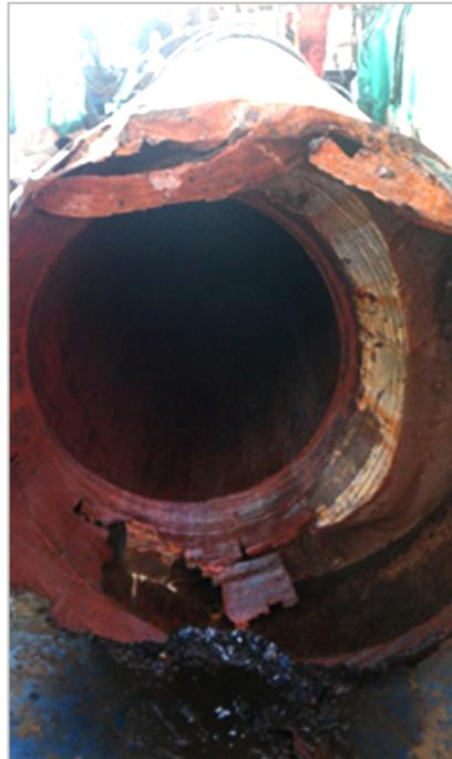
Successfully cut through cemented 13<sup>3</sup>/<sub>8</sub>-in. and 20-in. casing strings downhole.
