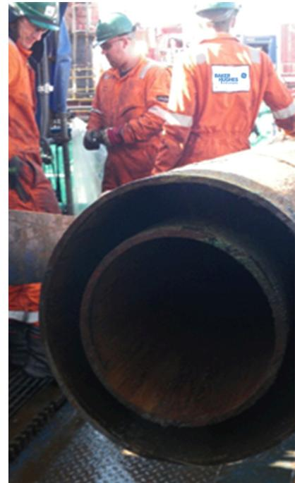
Successful cut 13<sup>3</sup>/<sub>8</sub>-in. and 20-in. dual-casing strings at surface.
