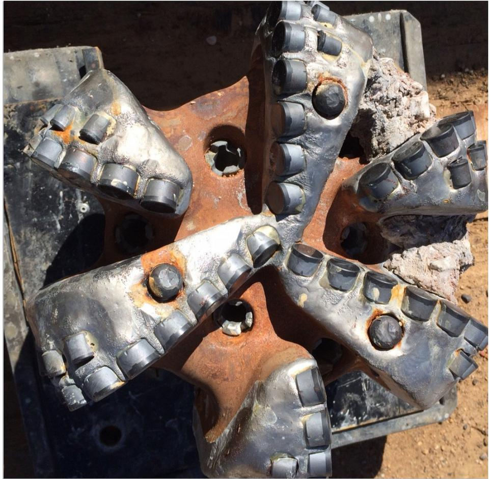
The TerrAdapt bit showed a very good dull condition after the run because its adaptive elements mitigated stick-slip and absorbed impacts to protect the cutters.
