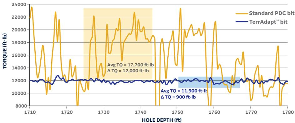
By automatically adjusting DOC control throughout the run, the TerrAdapt adaptive bit was able to mitigate vibrations to smooth out drilling performance, enabling a longer, faster run with consistently lower surface torque compared to an offset with a standard PDC bit.
